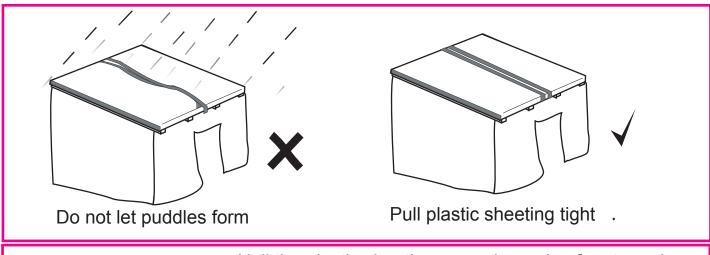
Nail the plastic sheeting around an edge for strength. Nail through the reinforcement bands if there are any.
