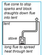
Chimneys usually pass through a metal plate attached to the tent roof, or a cement-fibre plate in the wall of the tent. Where no plates are available, chicken wire can be used.
